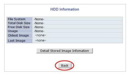
If **HDD Information** window displays all the fields as **-None-**, that means the hard drive is not in a formatted condition. To start formatting, click **Back** button to go back to the previous menu, and then click **HDD Status & Format**.
