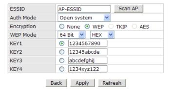
For WPASK or WPA2PSK, TKIP and AES can be available and the max length of encryption key is 63 digits of ASCII.
