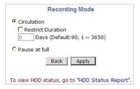
Now you are to choose the action between two options. If you want the FlexWATCH Server to keep recording without interruption, select **Circulation**. In this setting, the oldest file in HDD will be deleted first to make space for new video. If you want the FlexWATCH Server to stop recording and
