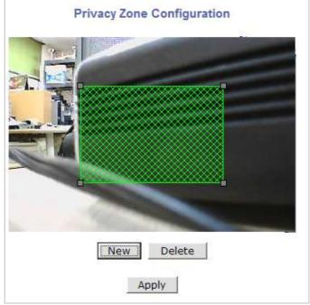
Privacy zone is marked with a rectangular shape. When you click **New** button, red-colored box will pop up and users can change its size and location. After that, click **Apply** button which will make box to green-color and finish the configuration.
