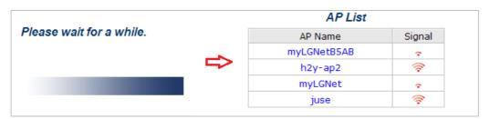
Note: Access points that are set to hide ESSID information for security won't be scanned by this method.
