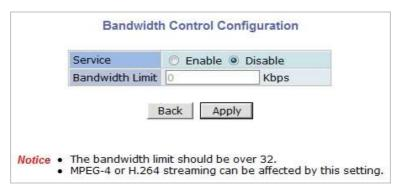
Note: This bandwidth control feature works fairly well in M-JPEG video transmission. But, for MPEG-4 and H.264, dropping data packets may cause low quality of video, so it is recommended to utilize CBR and frame rate control instead of bandwidth control for MPEG-4 and H.264 video.
