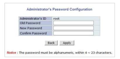
Default ID for admin account is fixed as "**root**" and not allowed to change. In **Old Password** field, enter the current password. In both **New Password** and **Confirm Password** fields, enter the same new password. The password must be between 4 and 23 alphanumeric letters. Click **Apply** button to put it into effect.
