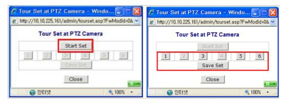
Select a Group number as desired, then click **Save Set** button to finish setup. The usage of Tour can be controlled at PTZ Control window in Smart Viewer.
