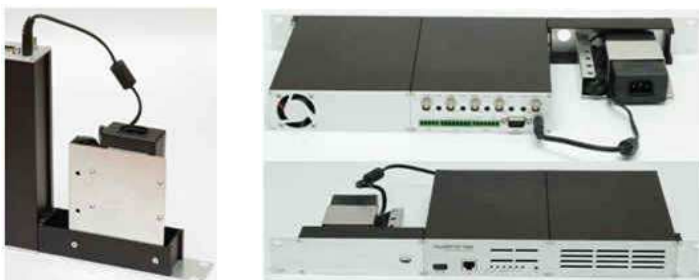
G. Plug Power cable to Power connector and finish installation
